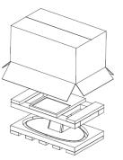
Step 4: Remove the Top End Pad from the top of the pedestal.
