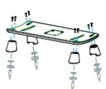
**Step 3:** If the combination spikes/glides were installed on the cradle, remove the spikes, felt washers, and knurled locking rings. If the combination spikes/glides were not installed, continue to Step 4.
