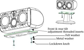
**Step 8:** Slide the loudspeaker in the cradle to adjust the tilt. When the loudspeaker has been appropriately positioned, firmly hand-tighten the tilt adjustment knobs to lock the loudspeaker in place. Do NOT over-tighten.
