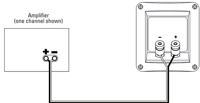
1. Connect both loudspeakers using the same method, using speaker cables of the same length for each speaker.
