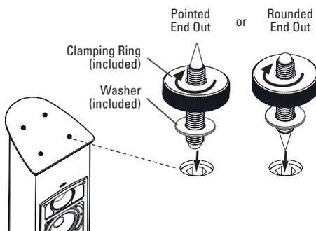
**NOTE:** When moving the F228Be with the spikes installed, avoid dragging the loudspeaker across the floor.
