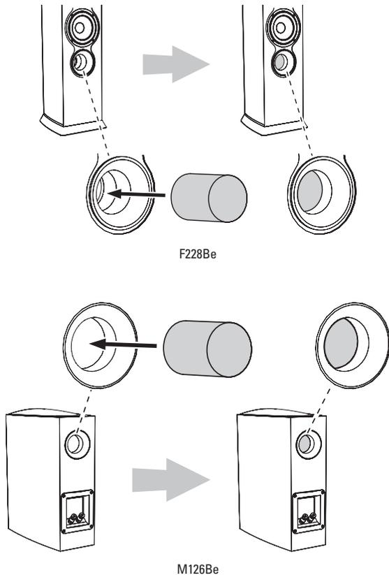
**CAUTION: Be careful not to insert the port plug so far into the port tube that it falls inside of the speaker.**
